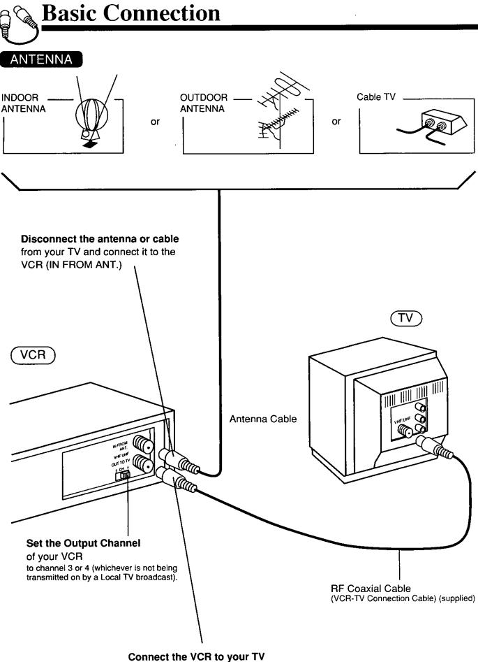
with the RF Coaxial Cable (OUT TO TV).
